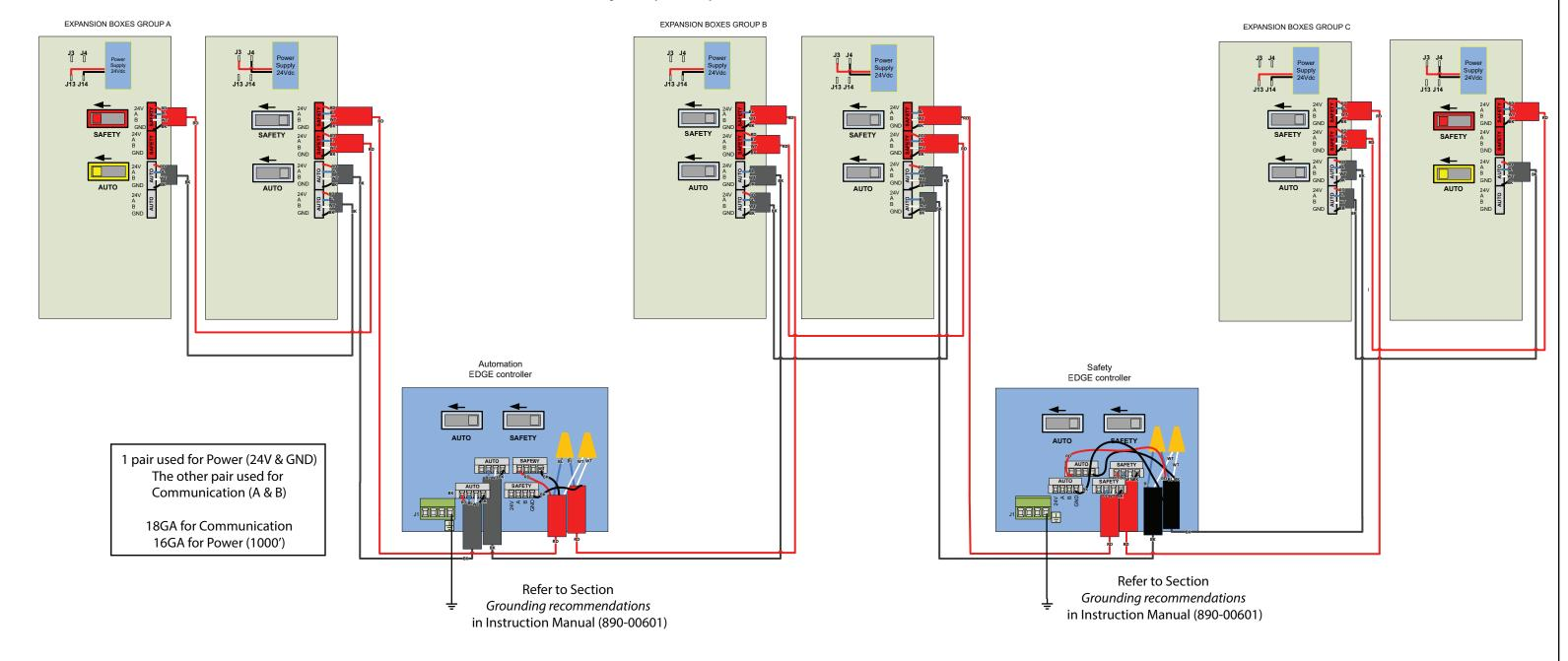
Shields ust be connected between all boxes (1 GND per communication bus) and must be connected to EARTH at one end of the circuit. NOTE: END OF LINE for communication: Red for Safety and Yellow for Automation Rules:
