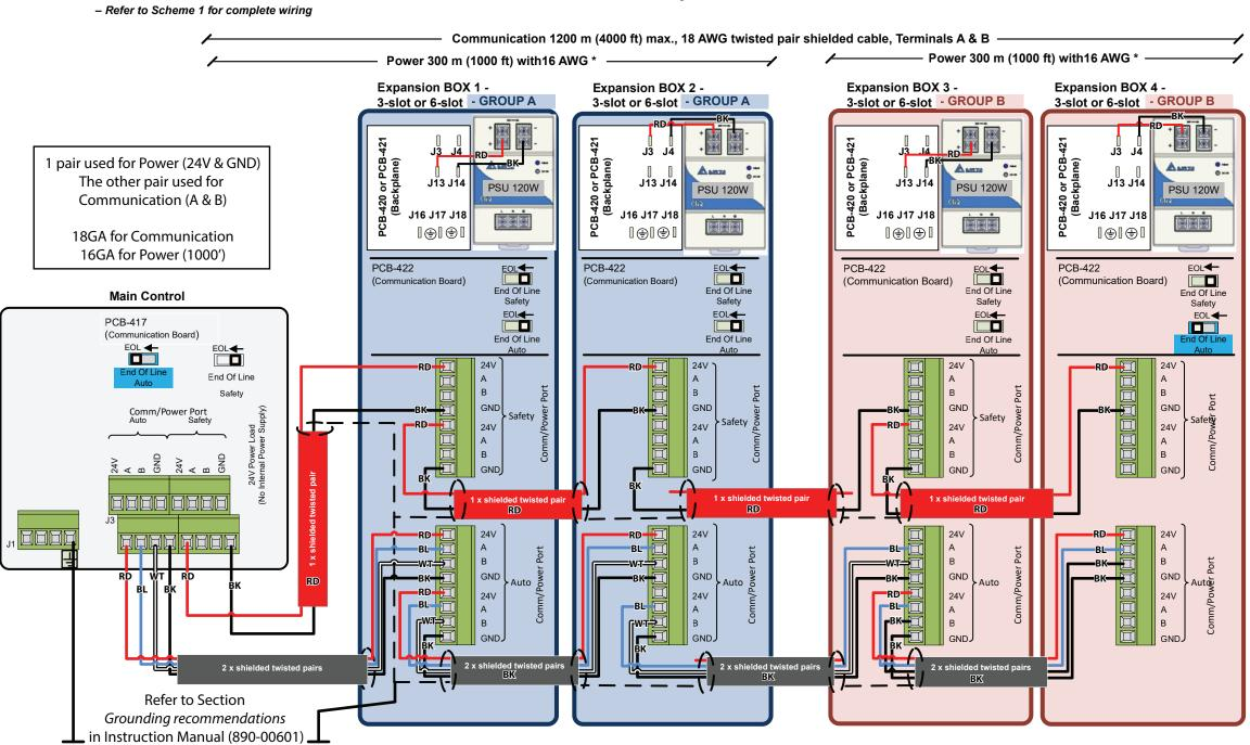
With even number of modules, redundancy power wiring is made by group of 2. In this example, GROUP A is in blue and GROUP B is in pink.
