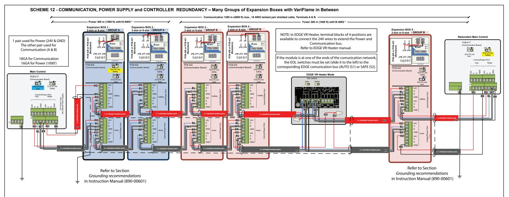
With odd number of modules, redundancy power wiring is made by a groups of 2 expansion boxes and 1 group of 3 expansion boxes. In this example, GROUP A is in blue and GROUP B is in pink.
