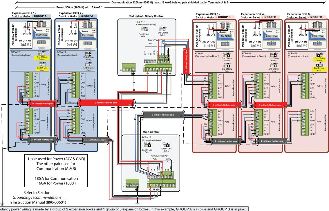
With even number of modules, redundancy power wiring is made by a group of 2 expansion boxes and 1 group of 3 expansion boxes. In this example, GROUP A is in blue and GROUP B is in pink. Rules:
